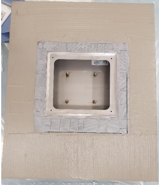
Image 3 – Mira 3690 One-seal on the front plate and Mira 4630 Aqua-flex 2K Membran on the plasterboard
