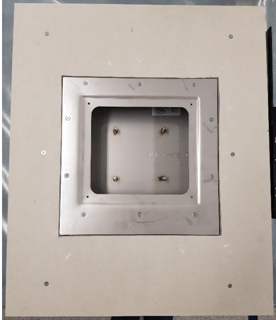
Image 2 – Mounting of Joramark Box300 in a plasterboard
