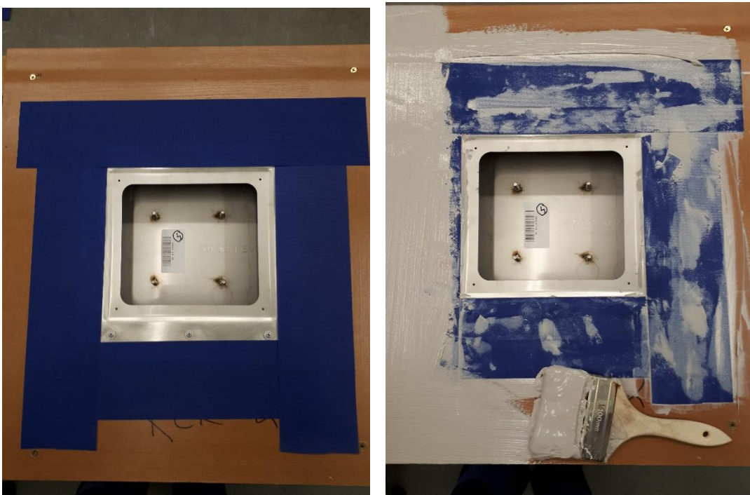
Picture 3-4. Preparation of test specimens Casco Waterproofing tape
