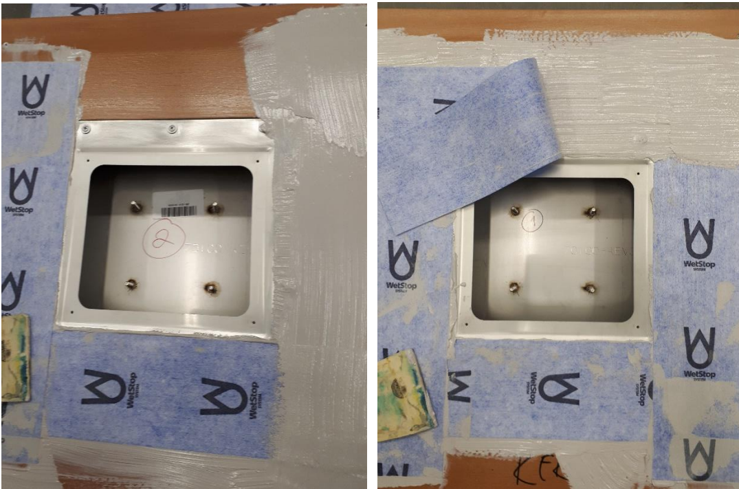
Picture 1-2. Preparation of test specimens WetStop KL-tape
