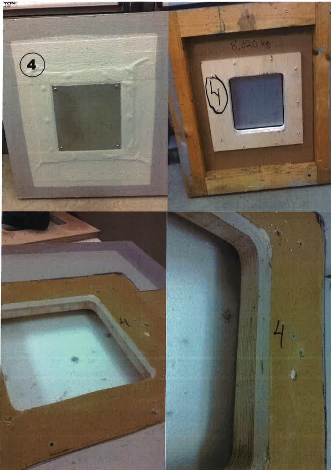
Picture 4. Test specimen no. 4 after testing.
