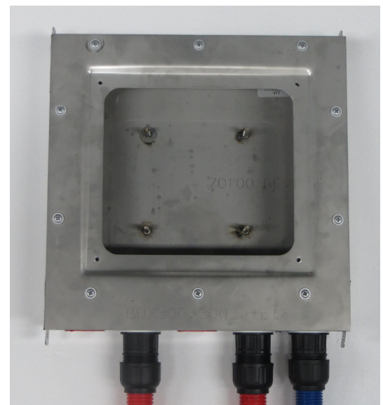
Fig.2. Test sample without a cover plate in the service opening, three bushings with protection pipes mounted.
